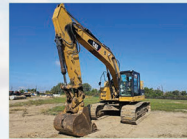
CATERPILLAR 328D LCR EXCAVATOR
