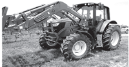
'19 John Deere 6110 M w/John Deere 620R Loader & Bucket, Cab, 4x4, 24x24 PQ Transmission, 24" Front, 34" Rear, 110 Engine HP, 261 Hrs., Same as New, #921066
