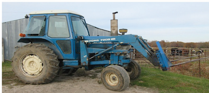
FORD 7700 Blue Power Special 90hp Tractor w/ Ford 7209 Quick Detach Loader (3 remotes, loaded, 540 or 1000 PTO) 5900 hrs
