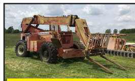
Traverse Extension Lift
