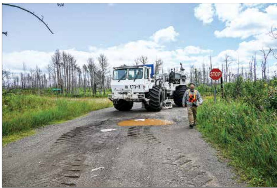
Jeff Hislop of Evergreen Geophysical walking in front of the 62,000-pound NodalSeismic vibroseis truck hired by Pulsar Helium to conduct a seismic survey along the Dunka River Road. photo by C. Clark
