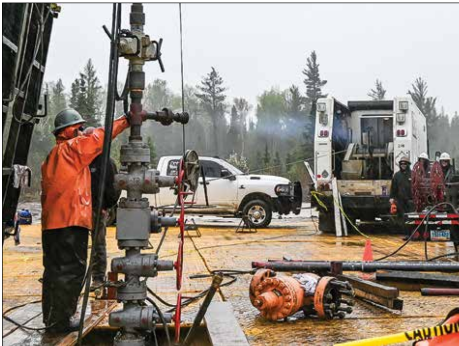
A slight blue haze shows the gas venting from Pulsar Helium's "exploration borehole" seconds after the flow valve was cracked open for the first time on the just completed well. photo by C. Clark
