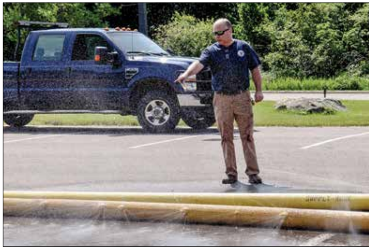
Ely Fire Chief David Marshall points at a large diameter fire hose that sprang multiple leaks during a pressure test on July 10. photo by C. Clark
