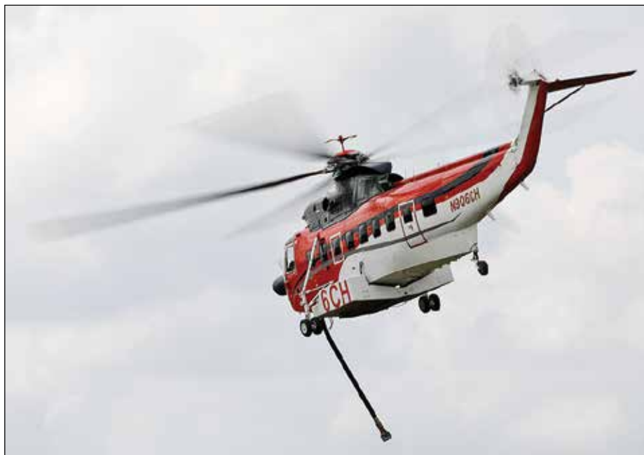
A refueled Sikorsky S-61 helicopter leaves the USFS Air Attack base at the Ely Airport last Friday to continue battling the Greenwood Fire. The helicopter can suck 1,000 gallons of water out of a lake or stream and dump it with pinpoint accuracy on a fire.
