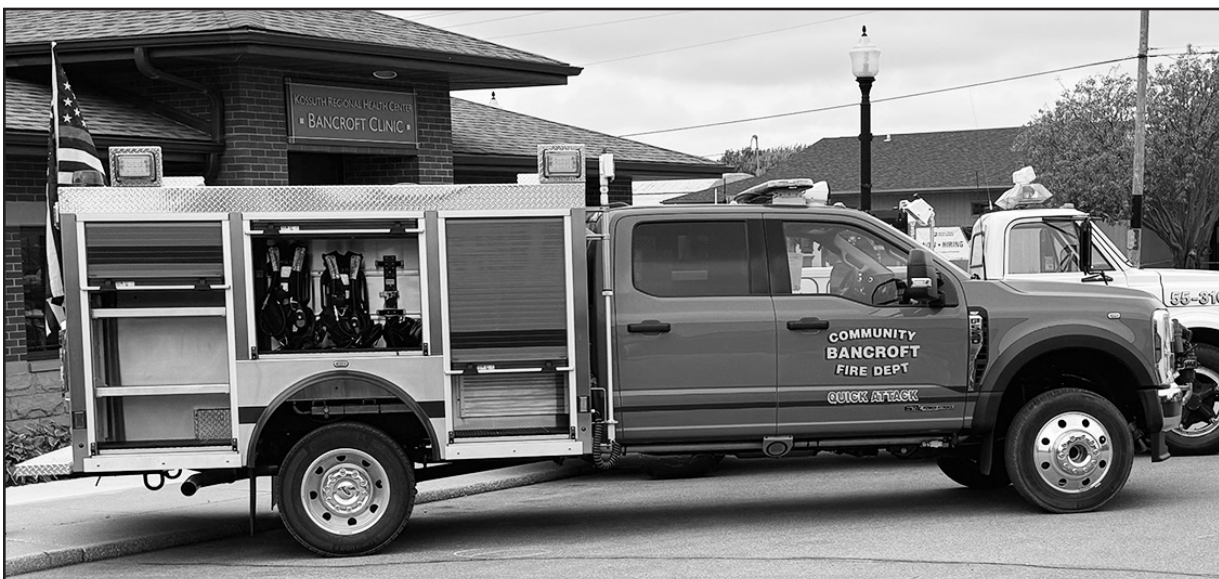
The Bancroft Fire Department has recently purchased four-passenger quick response truck, replacing the outdated 1969 Chevy grass rig, offering enhanced storage and a 300-gallon water tank with pump and front-mounted nozzle that can be controlled for inside the cab. Other upgrades in the past year have included a modernized SCBAs, a cylinder refilling station, and an upgraded water tanker truck with a portable drop tank and front mount nozzle. They have also acquired an advanced 'Jaws of Life' set from Hurst, featuring 100% battery power for expedited extractions.
