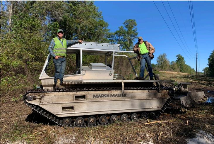
Top left: The Valentine family has a long history of working to improve properties and clear swamp power lines in Florida. The machines shown above are part of a system called the “Swamp Arborist,” which trims trees 45 to 75-feet in the air while floating along power lines through the swamps. The “Marshmaster,” a tractor-like machine, pulls a 25-foot airboat hull containing a remote controlled, all-terrain tree trimmer with a drum mulcher head. It was the first one in the United States.
