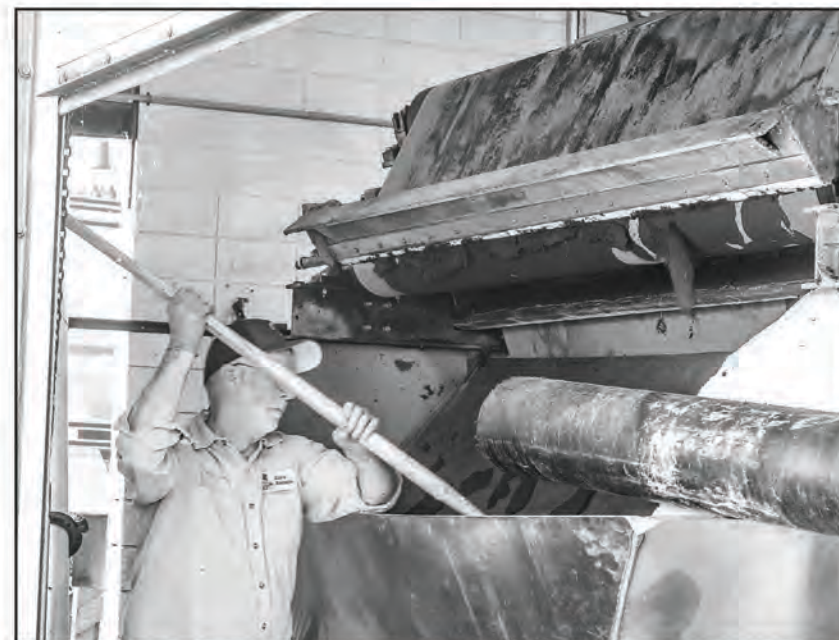
Walt scrapes "sludge cake" from one of the rollers used to press water from the mixture.
