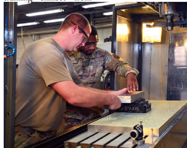
Master Sgt. Tyler Dickson and Senior Airman Shimon Hunt, 512th Maintenance Squadron, work on a C-130J Super Hercules egress door jettison bracket on Yokota Air Base, Japan, March 17, 2025. During their time at Yokota AB for annual tour training, Dickson and Hunt were part of a three-person team that researched and programmed specifications for the brackets.. (U.S. Air Force photo by Staff Sgt. Shavna Hodge)
