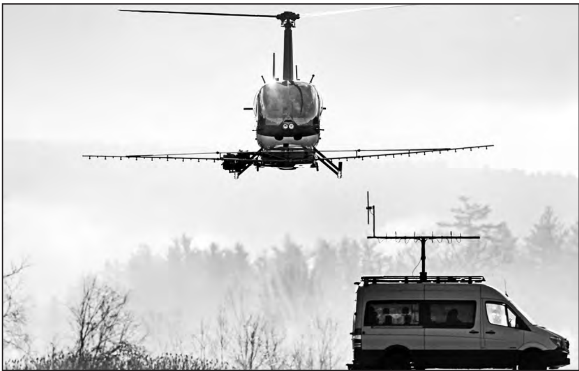
A Rotor Technologies unmanned semi-autonomous helicopter flies away from a van containing a ground control pilot/operator during a test flight over Intervale Airport, Nov. 11, in Henniker, New Hampshire.
